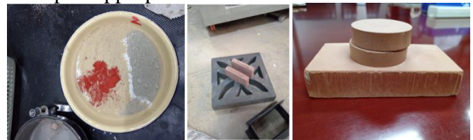
Fig.1. The process of producing ceramic bricks.
