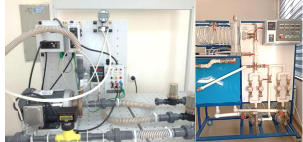
Fig.2. Laboratory installation of electric drive control with frequency converter of a centrifugal pump.
