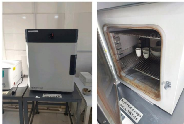
2-rasm. Angren IES kul namunalarini laborotriya sharoitida quritish uchun ishlatilgan quritish shkafi (Model: MST-55).
