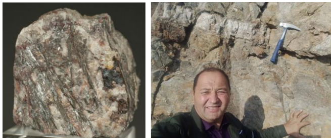
11-rasm. Vismutinni ignasimon kristallari bornit Cu_5FeS_4 (qora rangda) bilan.
