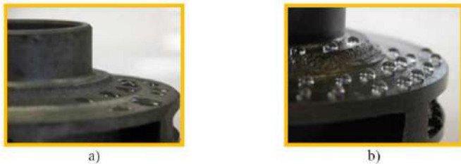
Fig.3. Impellers of a centrifugal pump: (a) original condition; (b) after modification using a hydrophobic coating.
