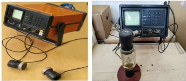
1-rasm. UK-10PMS defektoskopning tashqi ko'rinishi.
