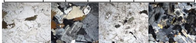
2-rasm. Bokali intruzivining asosiy fazasi jinslari: a, b — amfibol-biotitli tonalit (BK-78); d, e — amfibol-biotitli plagiogranit (BK-91); a, d — 1 nikolda, b, e — 2 nikolda; ko'rish maydoni 3,0 mm.
