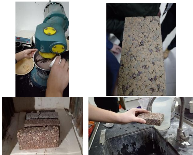
Fig.2. The process of producing ceramic granular permeable paving stones.
